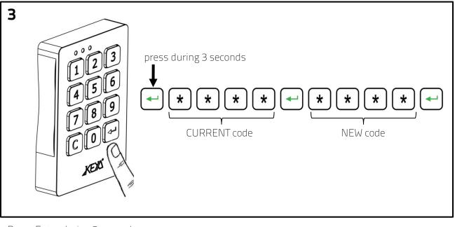
Press Enter during 3 seconds. Introduce Current code and press Enter. Introduce New code and press Enter.
