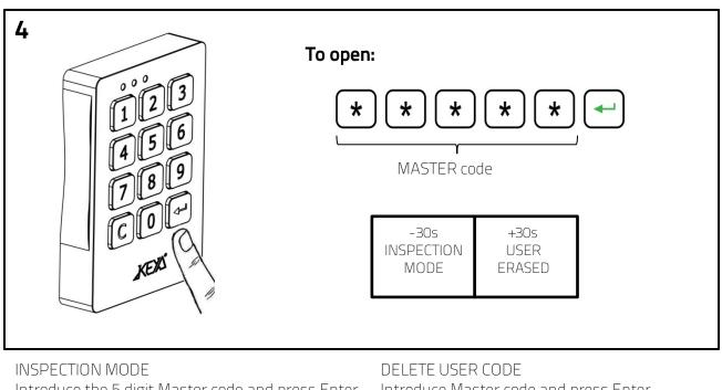
Introduce the 5 digit Master code and press Enter Close the lock by pressing Enter before 30s. The User code is not deleted.
